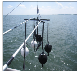
Polarimeter Instrument with three polarizer filters on the top of each radiometer oriented at 0,90 and 45 degree from reference horizontal
